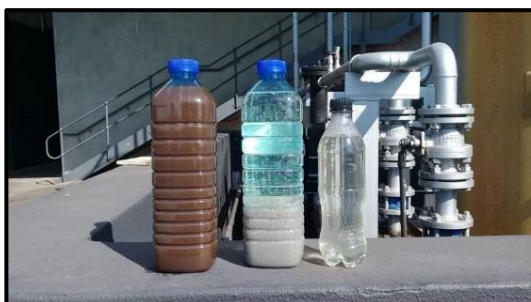
Figure 1: Before treatment, sludge removal and after removal.
