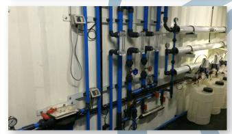
Containerized Underground Mine 1500 L/H RO System
